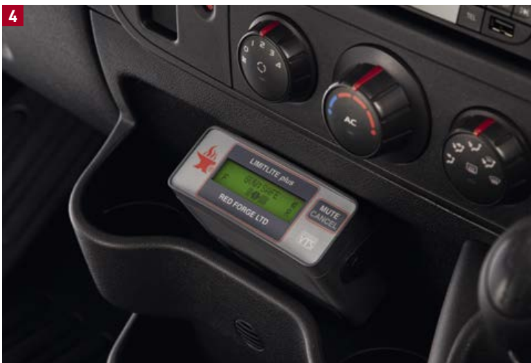
The Limitlite™ Plus system helps to ensure the vehicle is loaded to its maximum capacity improving profitability by reducing the wear and tear caused when running an overweight vehicle.
